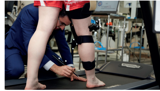
A patient at the research centre is put through their paces on the KneeKG video gait analysis machine by Alex Fuentes of manufacturers Emovi
